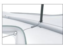
Step 8: Zip graphic closed around top of frame. Pull all cables out until inside loop is flush with eyelets. Attach all cables together at a single point for hanging.
