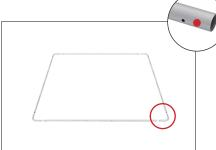
Step 7: Unzip print and place one frame inside. Position holes on frame to align with eyelets in graphic. Thread cable through eye let. Repeat for all eyelets.
